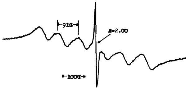
Fig. 2. ESR spectrum of \gamma -ray irradiated sample IV, treated with solution of potassium permanganate.
